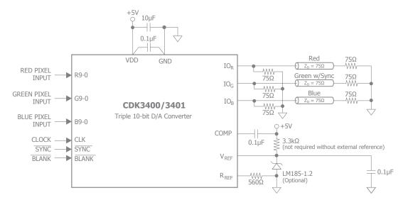
Figure 9. Typical Interface Circuit Diagram
