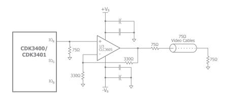
Figure 7. Graphics Output Driver Circuit Diagram
