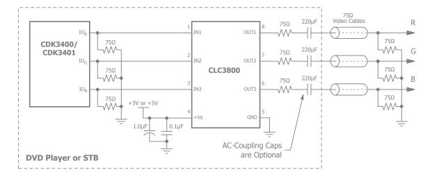
Figure 6. Standard Definition Video Output Circuit Diagram
