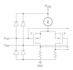
Figure 5. Equivalent Analog Input Circuit
