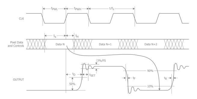
Figure 1. CDK3400/3401 Timing Diagram
