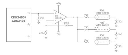
Figure 8. Standard Definition Video Distribution Circuit Diagram
